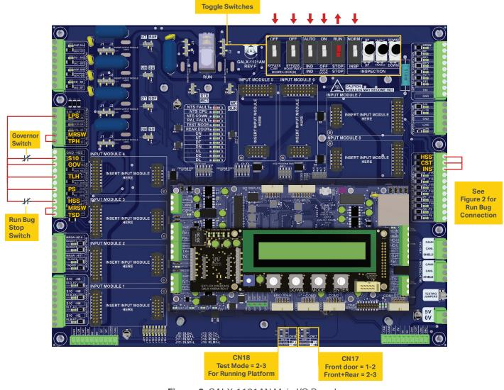
Figure 3: GALX-1121AN Main I/O Board
